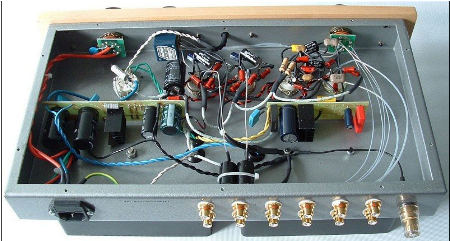
Basie Mk2 Complete. The circuit is more complex than the original srpp unit and more of a challenge to build. A little crowded with the extra tube socket and phono stage.
